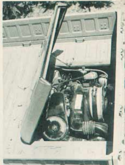
Trap door in the bed provides entry to the top of the engine and carb. Bed sides are removable.
