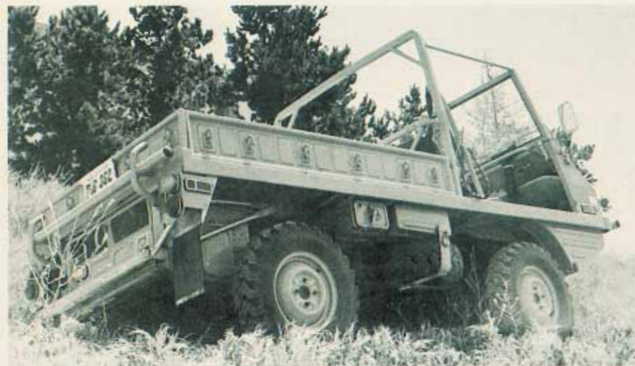
Spare tire carrier is well protected from road damage, and one can carry another spare on the opposite side. Canvas top support does double duty as a roll bar, and all detail work is really quite well done.
