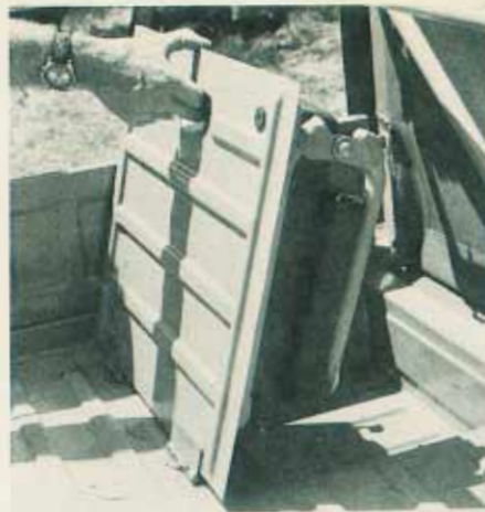
If needed the rear seats unfold like a jack-in-the-box from the flat bed floor. Seats move with ease, and it's a one hand operation.
