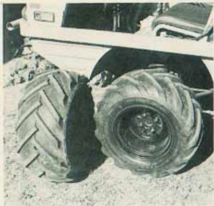
Terra tires and wide wheels are an extra that would be handy in the sand or swamps. Cabin drain plug, just visible above the tire, looks like a jacking point, but it is not. It is tricky to use a floor jack on the Steyr.
