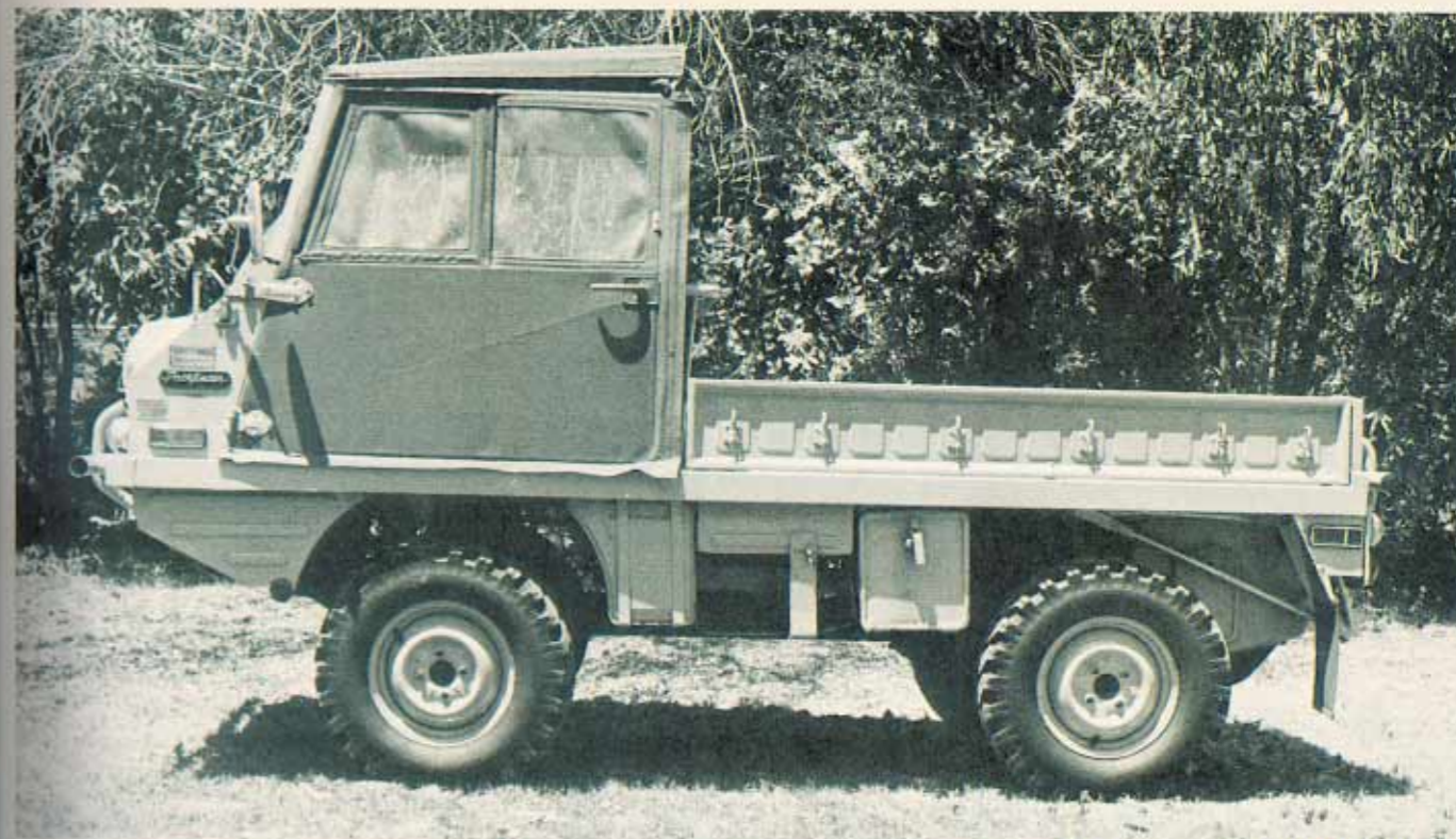
Short wheelbase is really visible from the side view; door/window piece just lifts out of the slot, and top is easily removed and replaced by using the tiny tie down tabs.
