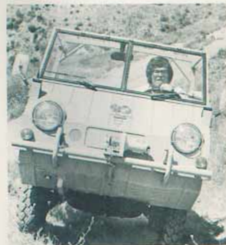
Head on the Hafflinger looks purposeful with street legal bumper and lights. Rubber topped brackets just inside the mirror mountings are stops for the windshield when it is folded down.
