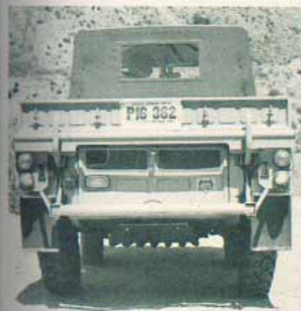
Lower rear bumper is a U.S. addition, mud flaps, all lights, including back up, are standard. Test unit had a towing plug (left), and engine is tucked in behind the screen.
