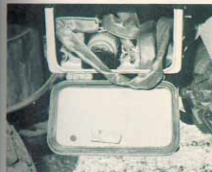
Storage bins carry the battery on one side, and the tool kits and miscellany on the other. All boxes are padlocked, and share a common key.
